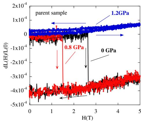
**Figure 3.** Isothermal magnetostriction  $dL(H)/L(0)$  of the parent sample as a function of the applied pressure at 4.2 K.
