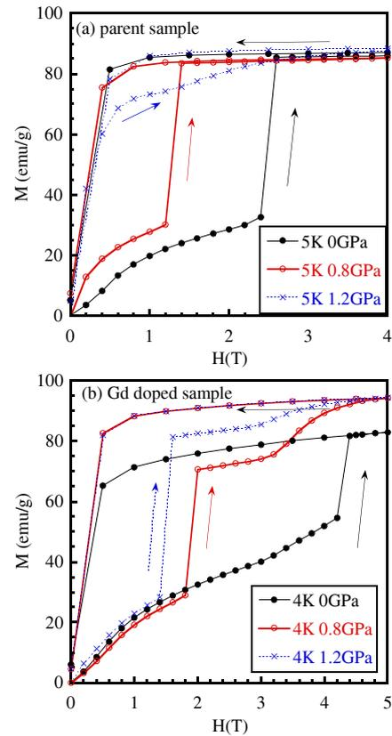
**Figure 2.** Isothermal magnetization curves measured under ambient and hydrostatic pressures after zero field cooling down to selected temperatures for both (a)  $\text{Eu}_{0.6}\text{Sr}_{0.4}\text{MnO}_3$ , and (b)  $(\text{Eu}_{0.9}\text{Gd}_{0.1})_{0.6}\text{Sr}_{0.4}\text{MnO}_3$  bulk samples. For each measurement, a magnetic field is applied up to a maximum field at the sweep rate of 0.2 T/step.
